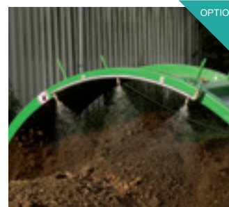
Water sprayer with nozzles. To achieve an optimal microorganism climate within the mound, the addition of water is essential.
