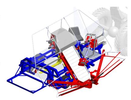
The machine is designed to harvest fruit into pallet boxes 1200x1000x760 mm. After mounting the bars, the platform for boxes and pallet's platform, it's possible to collect to boxes 600x400x150 mm.
