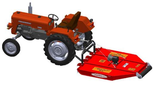
Using mower is possible by the symmetrical mounting as well as by a shift of axis of the tractor to the left or to the right side, depending on the model version. Cutting height is regulated by a back supporting shaft and the hydraulic tractor's lift.
