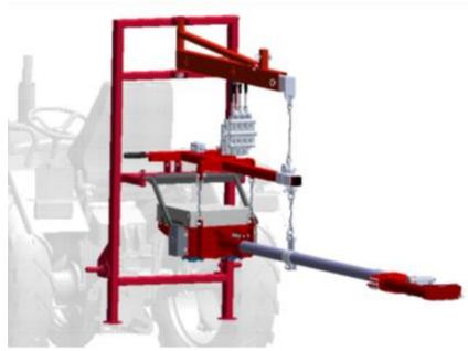
of the rotating components of shaking head. The length of the boom, on which hangs the shaker, is adjustable from 1200 to 2000 mm, makes it easier to work in the orchards of different row spacing.
