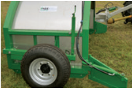
Hydraulic feeding plate, right side
