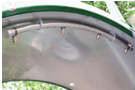
Water sprayer with nozzles. To achieve an optimal microorganism climate within the mound, the addition of water is essential.
