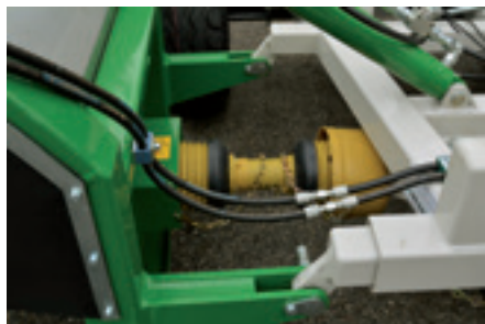
Direct drive – transmission on transfer shaft
