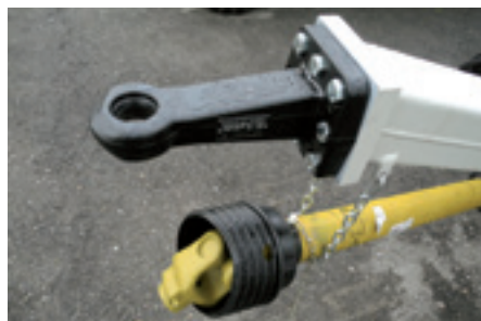
Standard trailer hitch front: DIN coupling
