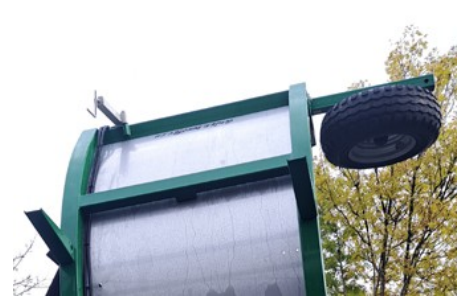
The jockey wheel can swivelled away for transport, no disassembly necessary.
