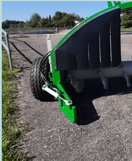
Hydraulic feed plate on the right
