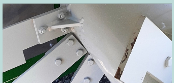
Long flails 260x80x15 - an advantage for heavy moving material
