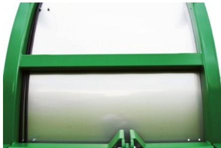
All wear plates are made of chrome steel.
