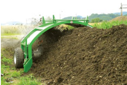
Maximum windrow size: 3.3 x 1.5m (TG 303), so that aerobic composting can take place.
