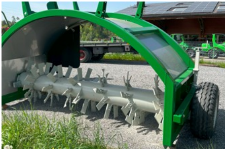
The solid arch construction made of 6 mm steel ensures very high stability.
